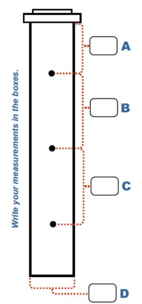
Take this measurement from the top of the post (not the top of the cap), to the center of the first hole.
